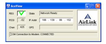
You can connect to your Raven locally or remotely using a known IP address or a fully qualified domain name. The display is updated periodically as AceView polls the Raven at a specified interval. *GPS is available only for PinPoint modems*.
